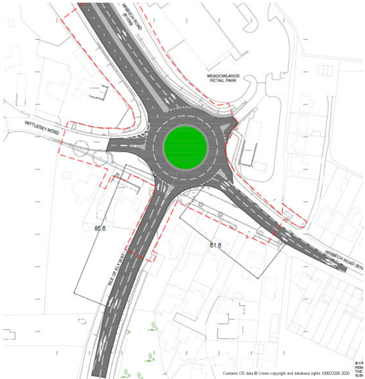
Figure 4.6: Peas Hill Roundabout Option 5.2 (50m ICD)
