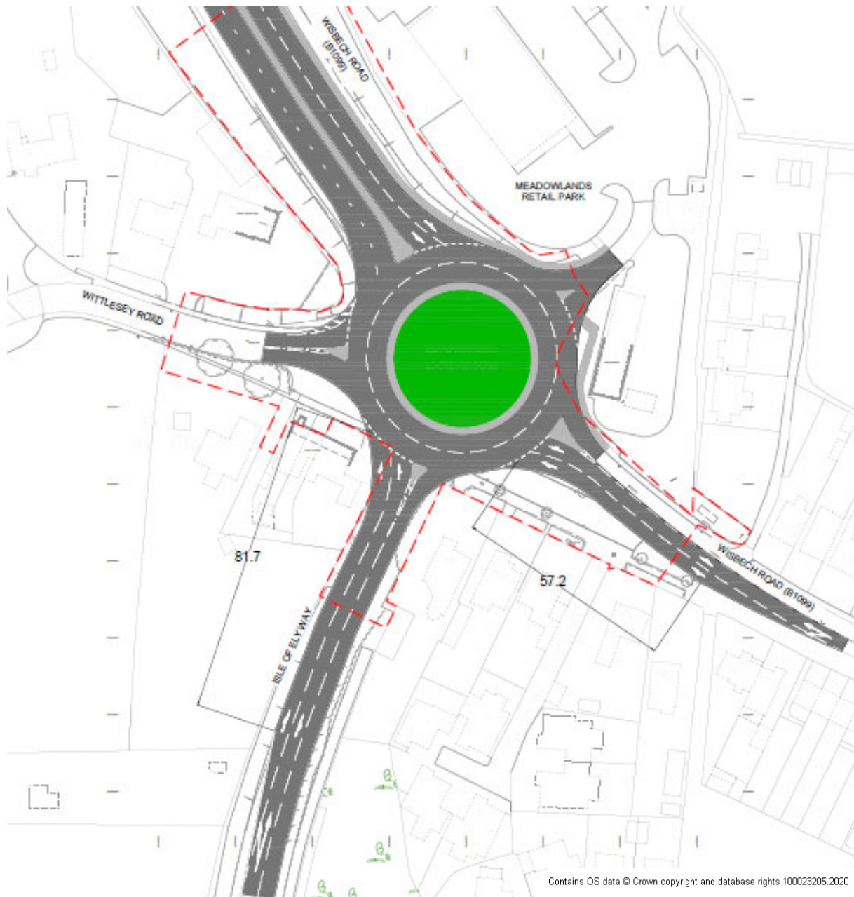
Figure 4.7: Peas Hill Roundabout Option 5.2 (60m ICD)
